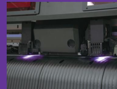
Applies UV-curable ink that hardens immediately through irradiation of ultraviolet (UV) light
